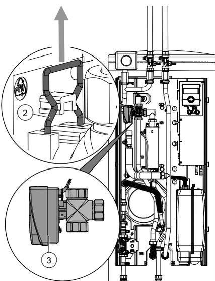
4. Carefully pull the valve motor (③) forward off the 3-way switching valve (④).
