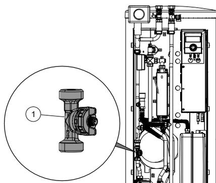
The volumetric flow meter / heat meter measures flow and temperature difference in the charging circuit. The measuring ranges are set in the heating and heat pump controller. Measured values can be read out on the control panel display.
