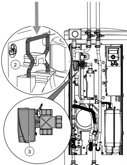
11. Ensure that the U-clip has latched into position correctly:
