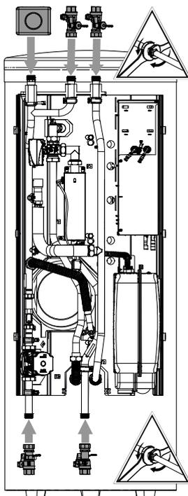
2. Lay the safety discharge of the safety valve into the drain via a funnel waste trap according to the relevant standards and guidelines. It is essential that the safety discharge is connected.
