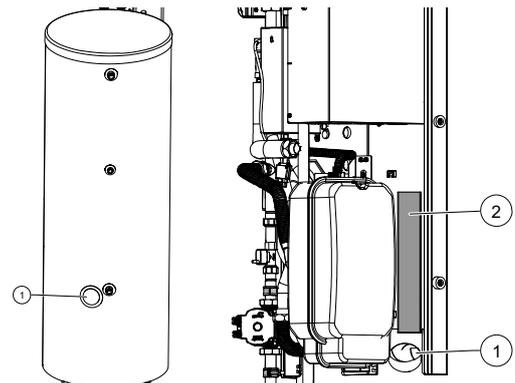
2. Feed the cables through the cable duct (2) to the switch box.
