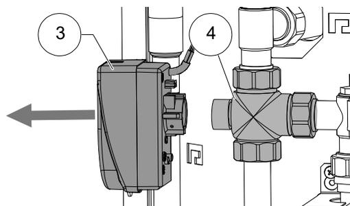
5. Turn the spindle of the 3-way switching valve so that the rounded side of the spindle points in the direction of marking A of the connections of the 3-way switching valve.
