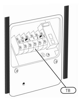
Communication is connected on terminal block TB.
