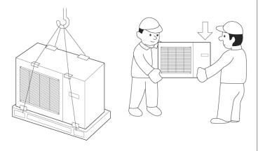
If L...Split needs to be transported across soft ground, such as a lawn, we recommend that a crane truck is used that can lift the unit to the installation location. When L...Split is lifted with a crane, the packaging must be undamaged and the load distributed with a boom, see the illustration above.
