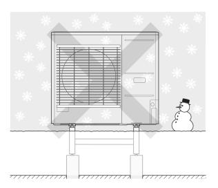
Prevent snow from building up and covering the grilles and drain holes on L...Split.
