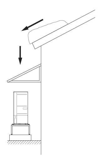
If there is a risk of snow slip from roof, a protective roof or cover must be erected to protect the heat pump, pipes and wiring.
