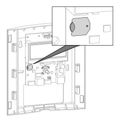
2. Dispose of the buffer battery according to local regulations.
