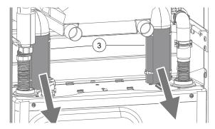
6. Remove 3 clips (④) on the hydraulic connections.
