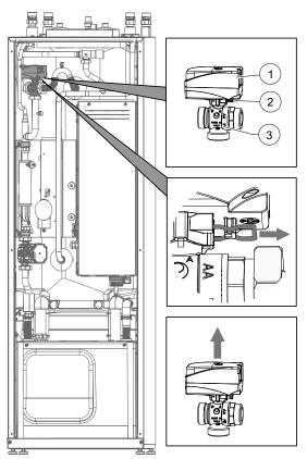
Turn the spindle (④) of the 3-way switching valve so that the rounded side of the spindle points in the direction of marking A of the connections of the 3-way switching valve.
