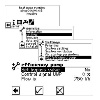
The "Set bypass valve" menu item is set by default to "No". The overflow valve adjustment function is deactivated.
