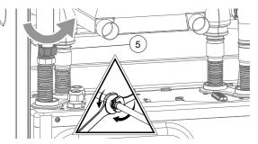
8. Disconnect the hydraulic connections; to do this, push the pipes (⑥) apart as far as necessary.
