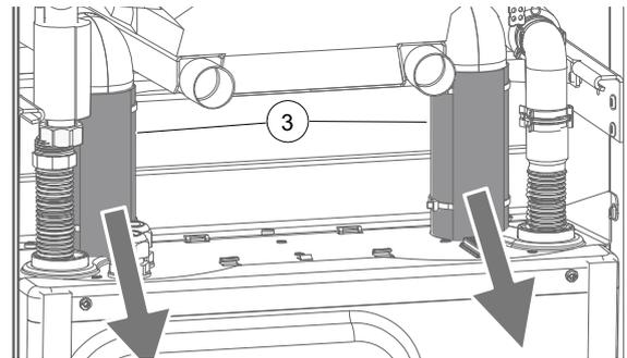
6. Remove 3 clips (④) on the hydraulic connections.
