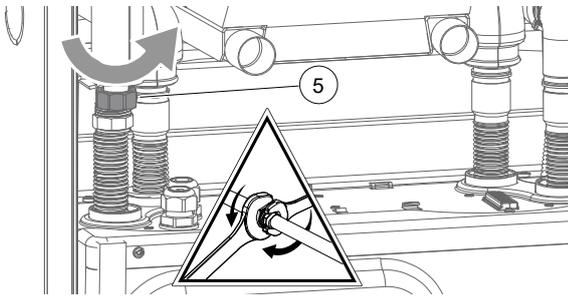
8. Disconnect the hydraulic connections; to do this, push the pipes (⑥) apart as far as necessary.
