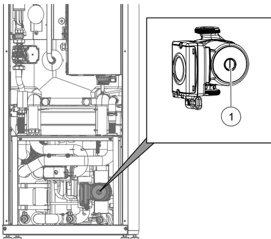
3. Insert a screwdriver into the opening and release the blocked shaft in the direction of rotation of the circulating pump.
