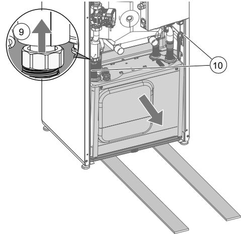
12. Slowly and carefully pull out the module box by the carrying lugs (⑩). Ensure that none of the pipes are damaged
