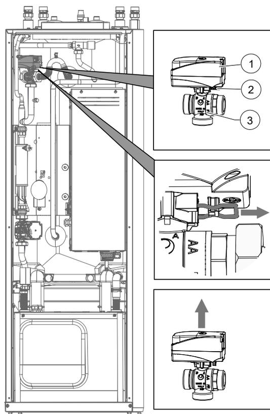
3. Turn the spindle (④) of the 3-way switching valve so that the rounded side of the spindle points in the direction of marking A of the connections of the 3-way switching valve.
