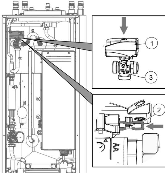
9. Ensure that the U-clip has latched into position correctly:
