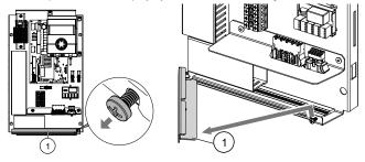
Route the wired plugs of the heat pump bus cable
